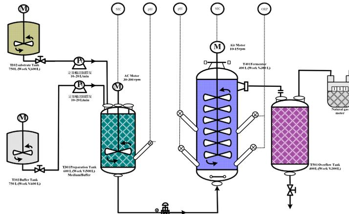
Figure 1 The layout of the 0.4 m<sup>3</sup> hydrogen production pilot plant
